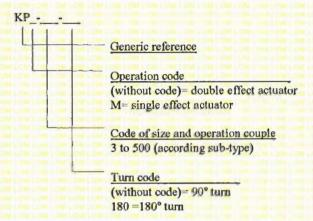
Single effect actuators (types KPM. ..) include recovery springs in variable quantity in each model.
